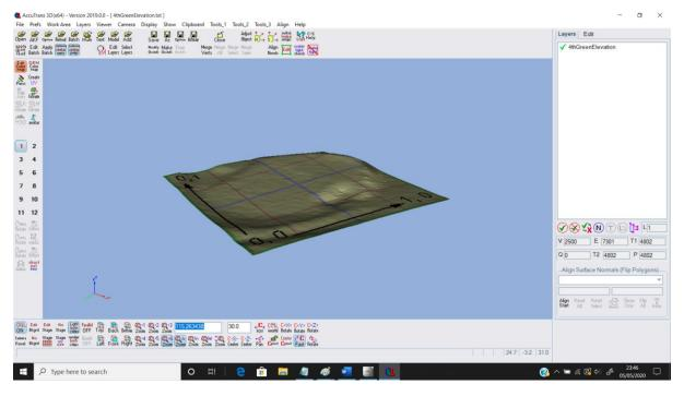
We now need to Save with Options as DXF, remembering to offset the centre by the co-ordinates used above. Click on 'Adjust' and enter the coordinates as negative values X = -595, Y = -540.
