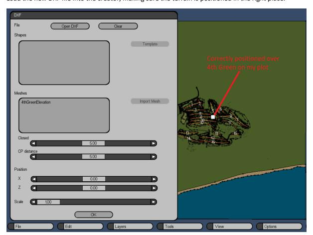
In the Height Layer we should now see that the green has been replaced with fresh terrain. The error has been fixed, but we will have to re-do the bunker, which has been flattened out. It is hard to see from the screenshot, but there is also a slightly steeper slope to a shelf at the back of the green, which is a consequence of the better resolution data on the green.
