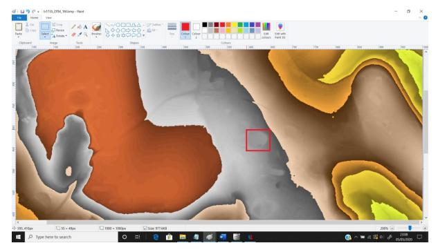
Because the LIDAR elevations start from the South West corner of the tile, while MS Paint Coordinates start from the North West corner, we need to subtract the Y co-ordinates from 1000, so the SW corner is at 595, 540 and the square is 50x50.
